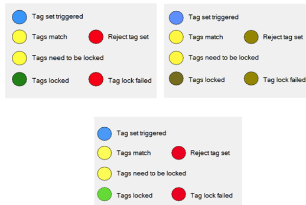
Figure 4. An example of what non-colorblind people see (top left) in a piece of software that the author developed, what people with deuteranopia see (top right) and a better choice of colors (bottom)
